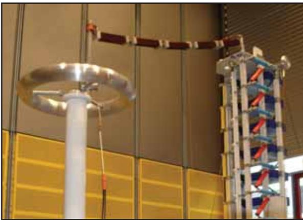
ERITECH Isolated Downconductor being tested
