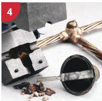
Open the mold and remove the
