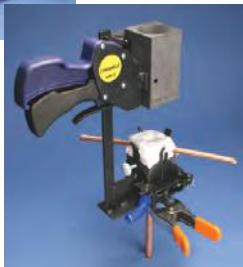
**Step 1:** Layer batting and variable conductor sizes to be welded into dry mold.
