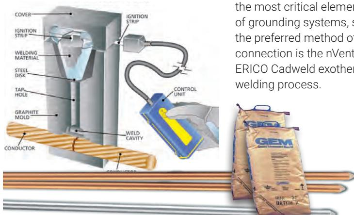
Connections are often the most critical element of grounding systems, so the preferred method of connection is the nVent ERICO Cadweld exothermic welding process.
