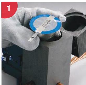
Insert Cadweld Plus cup into mold
